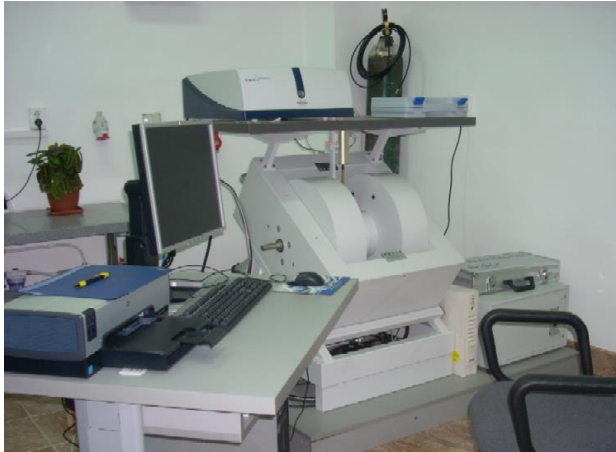
Electron Paramagnetic Resonance spectrometer Bruker EMXmicro, X band, variable temperature unit (ER4141VT)
