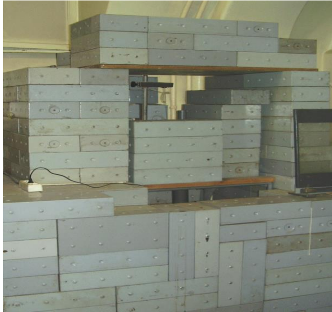
The irradiation facility with Am-Be (5 Ci), and Pu-Be (33 Ci) neutron sources. Fluence = 6.6 \cdot 10^7 n/s
