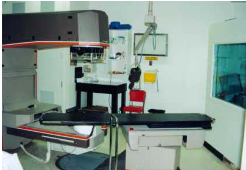
FIG. 7.5. A Conventional treatment simulator has capability to reproduce most treatment geometries available on radiotherapy treatment units. Simulators use a diagnostic X-ray tube and fluoroscopic system to image the patient.
