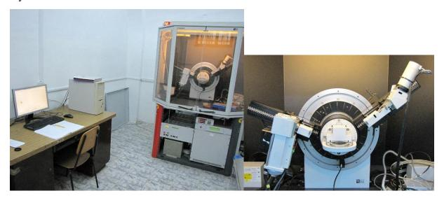
Within the Ioan Ursu Institute we maintain and staff an X-ray diffraction laboratory, equipped with a D8X Advance X-ray diffraction equipment from Bruker (XRD). We can collect high quality data for a wide range of analysis objectives, including:
