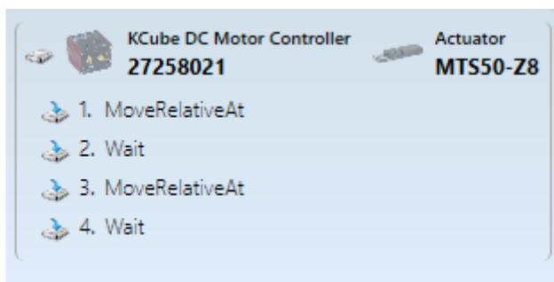
Figure 2.9. The command sequence for the linear actuator
