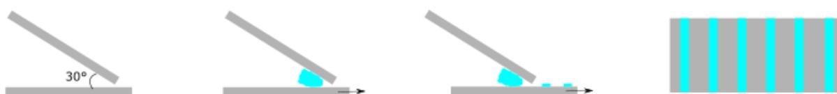
Figure 2.6. A schematic representation of the stop-and-go CSA method
