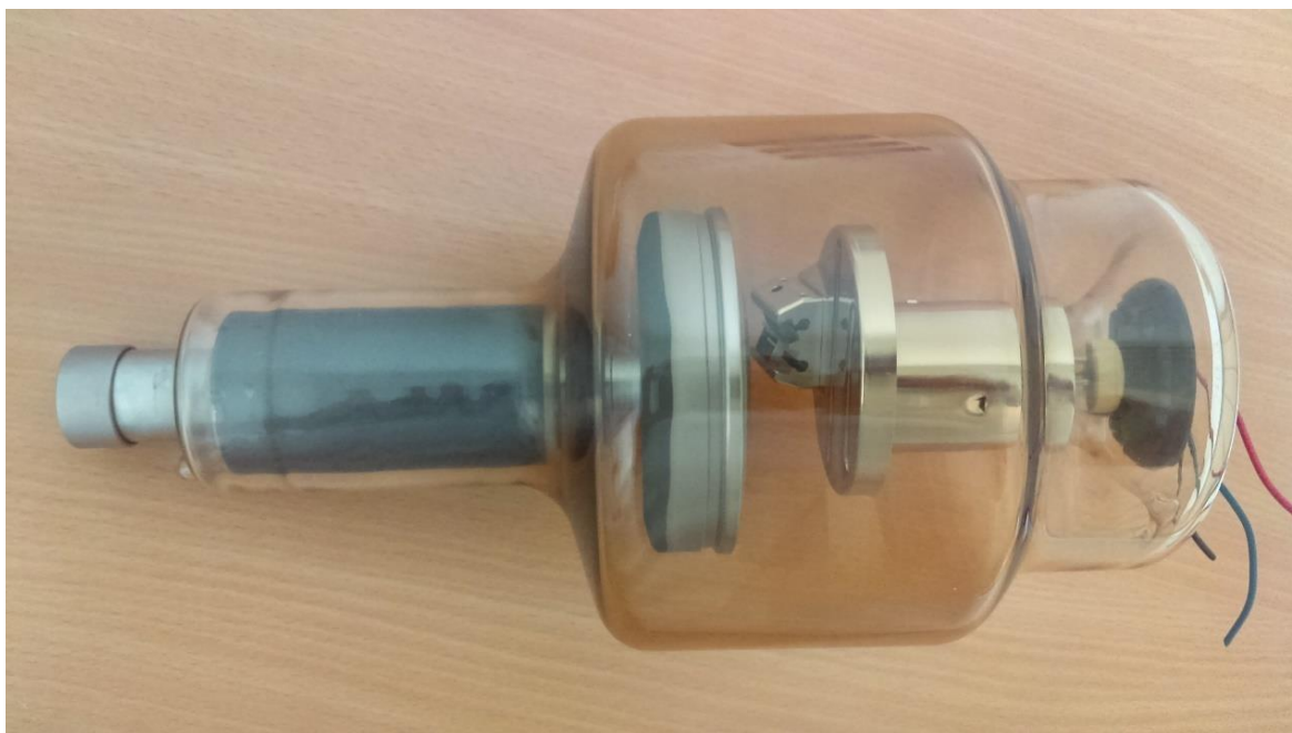
Fig. I.5.3 Tub RX de la aparatul CT SOMATOM DEFINITION AS
