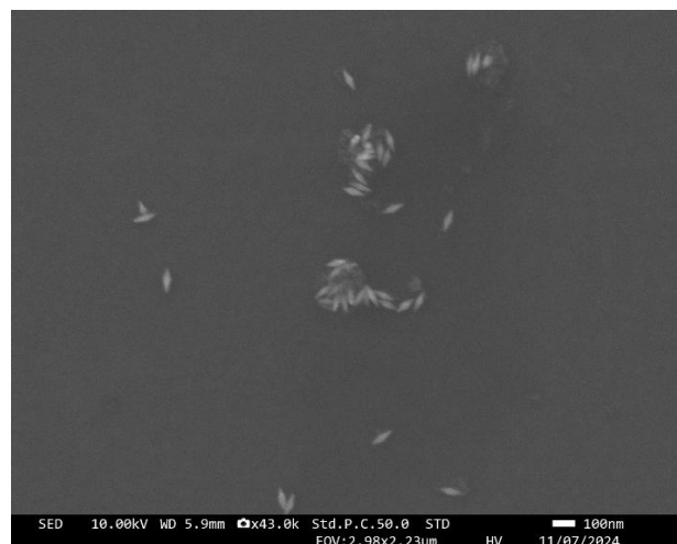
Figure 2.8 Left extinction spectrum of AuBPs synthesized with 40 \mu\text{L} of IS and right their corresponding SEM image
