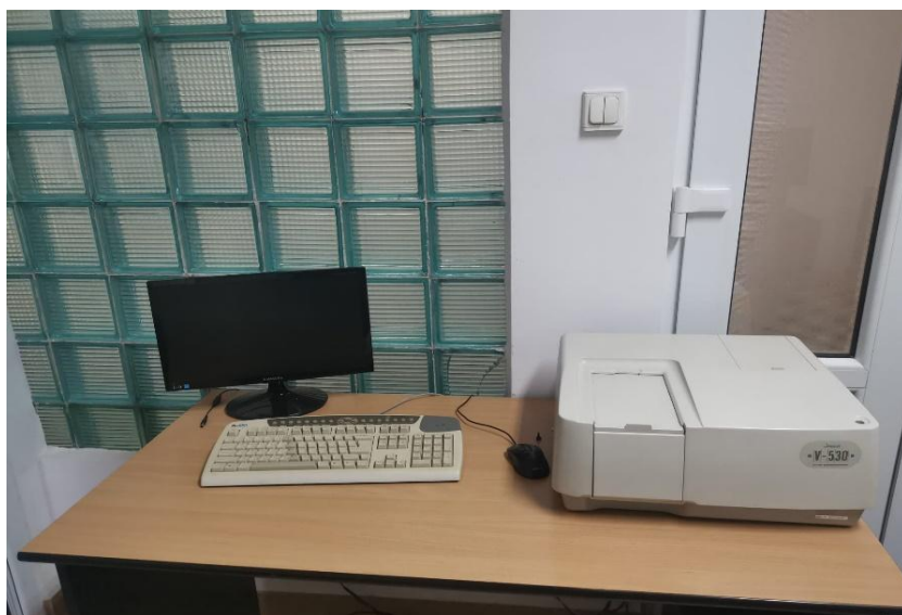
Figure A1.1 The spectrophotometer used for the absorption spectra
