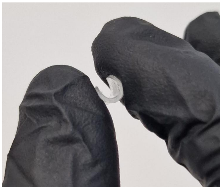
Figure 3.1 Image of transparent and flexible PDMS substrate that was used in this chapter
