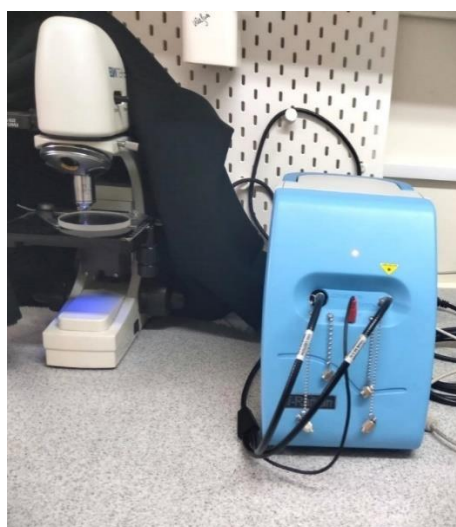
Figure 2-3 Portable Raman spectrometer (iRaman 532 nm, BWTek) with built-in laser and detector (right), coupled to a BWTek microscope with a 20x objective for focusing the laser on the sample (left).
