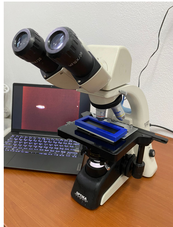
(b) The microscope is connected to a laptop, and the sample is digitized through the microscope's camera. Under the microscope objective, the black tape fixed to the blue frame is now marked with holes burned by the laser.
