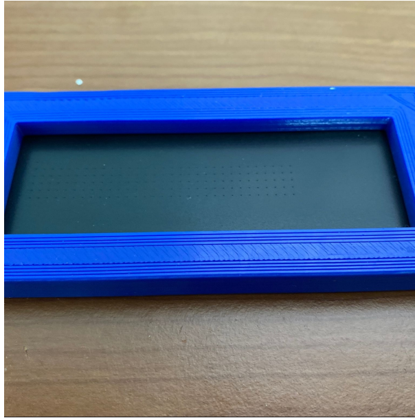
3.1. Figure. Holes burnt into the black tape fixed to the frame at different Z heights.
