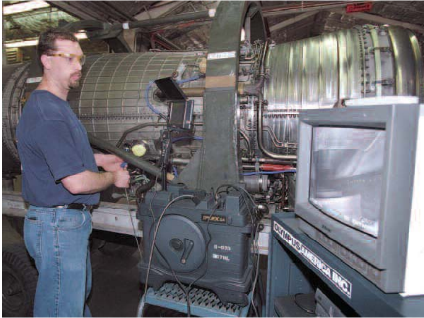
An Inspector at Tinker Air Force Base Gets a Magnified View of an Engine's High-Pressure Turbine Area with a New Digital Fiber-Optic Borescope. (Photo Courtesy of US Air Force; Photo taken by Margo Wright)
