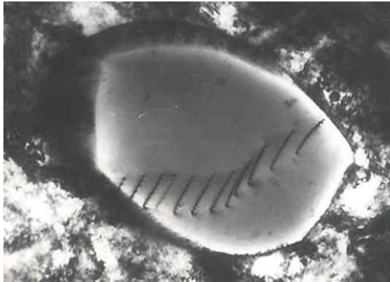
Transmission electron micrograph of dislocations
