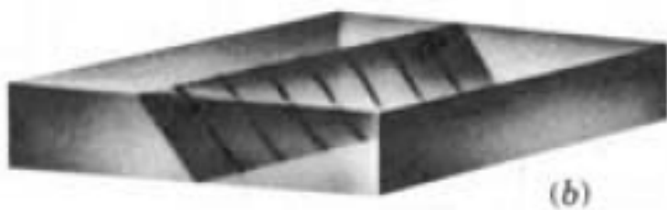
FIGURE 2.13 Observation of individual dislocations in thin foil. (a) Planar arrays of dislocations in 18Cr-8Ni stainless steels (from Michalak, 10 Metals Handbook , Vol. 8, copyright American Society for Metals, Metals Park, OH, 1973; used with permission); (b) diagram showing position of dislocations on the glide plane in the foil (after Hull 11 ).
