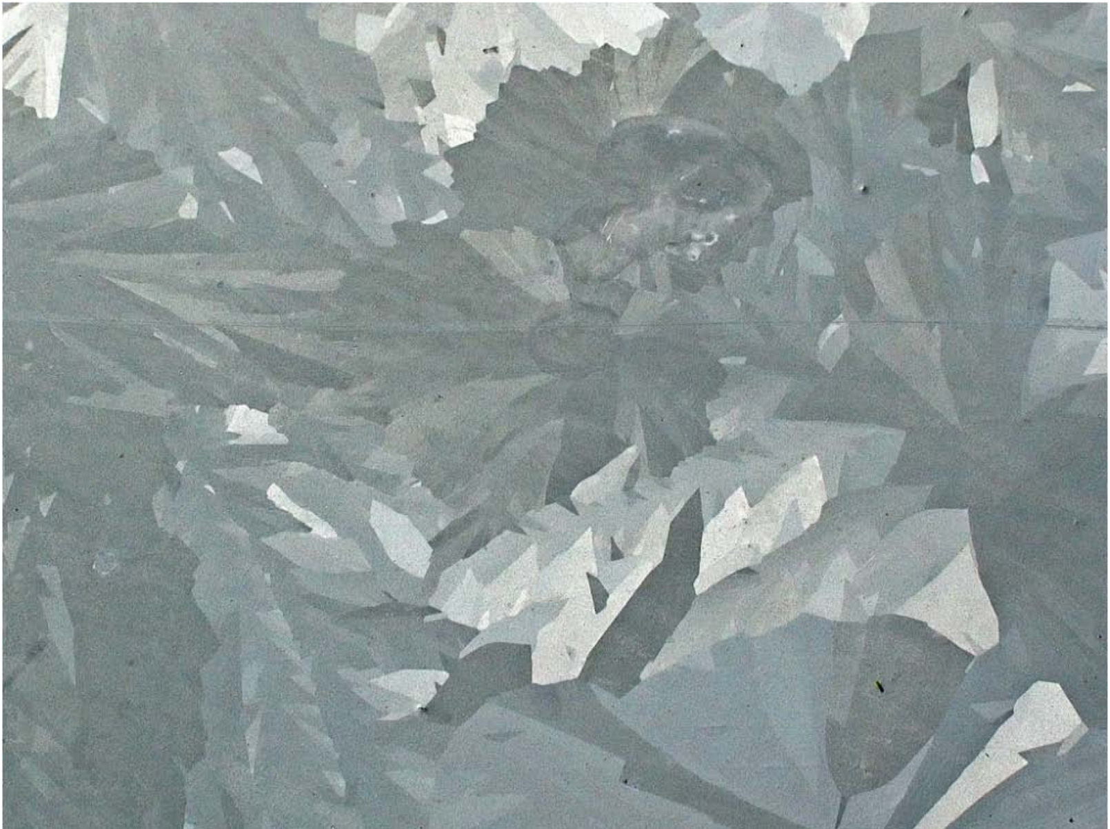
galvanized surface with cristallites of zinc
