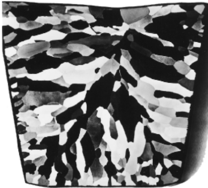
FIGURE 4.10 High-purity polycrystalline lead ingot in which the individual grains may be discerned.
