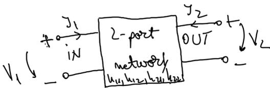
$$\begin{pmatrix} V_1 \\ I_2 \end{pmatrix} = \begin{pmatrix} h_{11} & h_{12} \\ h_{21} & h_{22} \end{pmatrix} \begin{pmatrix} I_1 \\ V_2 \end{pmatrix}$$
