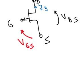
$$V_{GS} = 0 \Rightarrow I_D = I_{DSS}$$
