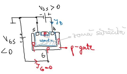
$$I_D = I_{DSS} \left(1 - \frac{V_{GS}}{V_T}\right)^2$$
