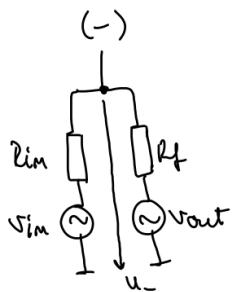
$$u_+ = \frac{\frac{V_{in}}{R_{in}} + \frac{V_{out}}{R_f}}{\frac{1}{R_{in}} + \frac{1}{R_f}} = \frac{\frac{V_{in}R_f + V_{out}R_{in}}{R_{in}R_f}}{\frac{R_f + R_{in}}{R_{in}R_f}}$$
