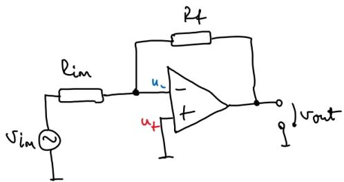
$$V_{out} = f(V_{in}, R_{in}, R_f)$$
