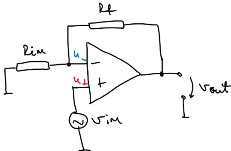
$$V_{out} = f(V_{im}, R_f, R_{im})$$
