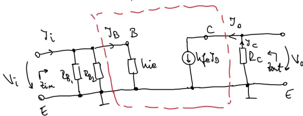
$$z_{in} = R_{B1} \parallel R_{B2} \parallel h_{ie}$$
