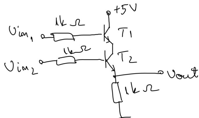
$$\begin{aligned} V_{in_1} = 0 \Rightarrow T_1 \text{ blocat} \\ V_{in_2} = 0 \Rightarrow T_2 \text{ blocat} \end{aligned} \quad \left\{ \Rightarrow V_{out} = 0 \right.$$
