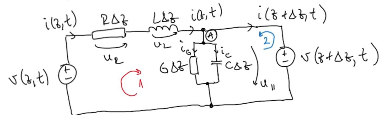
Ochiul 1:  $v(z, t) - i(z, t) \cdot R\Delta z - L\Delta z \frac{di(z, t)}{dt} - v(z + \Delta z, t) = 0$   $\left| \begin{array}{l} \\ \frac{1}{\Delta z} \end{array} \right.$
