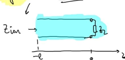
$$Z_{im} = \frac{V(-l)}{I(-l)} = \frac{V_0^+ (e^{jl\beta l} + r e^{-jl\beta l})}{V_0^- (e^{jl\beta l} - r e^{-jl\beta l})} Z_0 =$$
