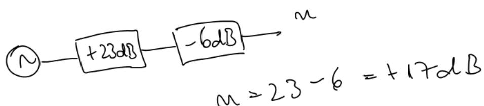
Pentru tensiuni  $m = 20 \log \frac{V}{V_{\text{ref}}} \quad (\text{dB})$
