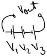
$$V_{out} = V_1 - V_2 + V_3 =$$
