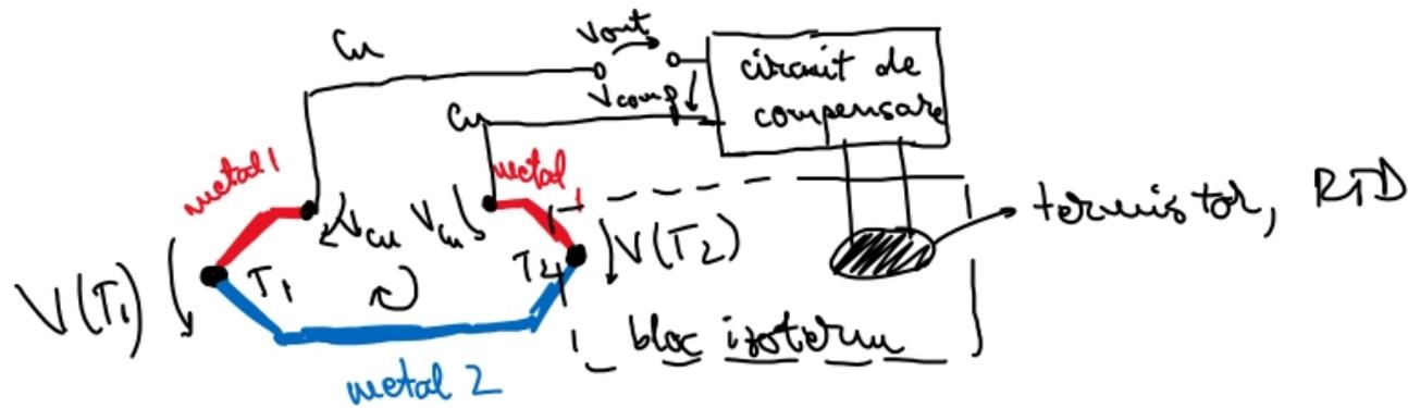
$$V_{out} + V_{comp} + V_{Cu} + V(T_2) - V(T_1) - V_{Cu} = 0$$
