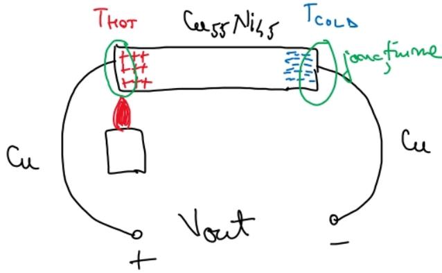
$$\Delta V = \int_{T_{COLD}}^{T_H} S(T) dT$$
